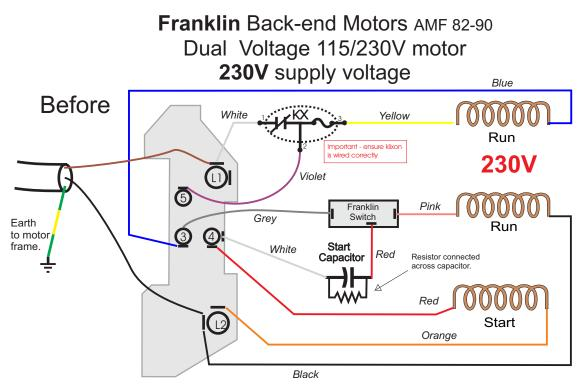
Note: The terminal positions may vary from that shown on AMF diagrams. These drawing are based on an actual motor from an 82-90XL
